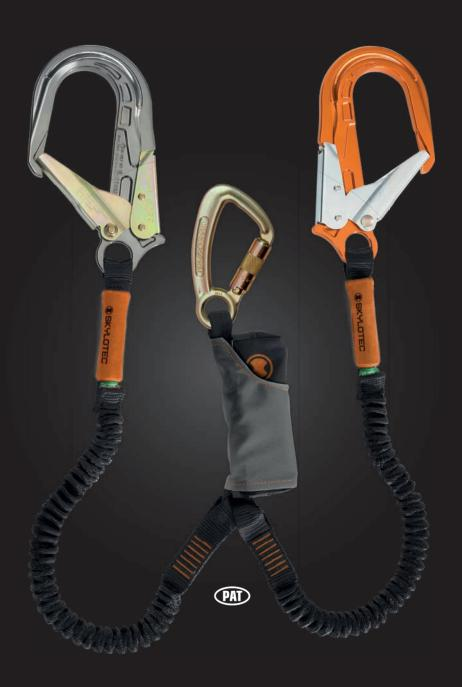
The **SKYSAFE PRO FLEX TWIN** lanyard range is the only twin lanyard on the market today designed specifically to avoid cross loading when used unintentionally e.g. when the unused lanyard is incorrectly attached to a HIP (Pole Strap) D-ring. This UNIQUE design feature results in the unused lanyard sliding down the deployed shock absorber. This avoids the possibility of the fallen person left partially suspended from the incorrectly positioned unused lanyard.
