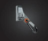
Removable stainless steel Type 1 fall arrest device for use on 12mm ropes. A dual redundant closing mechanism prevents the SKA device from being put on the rope incorrectly.
